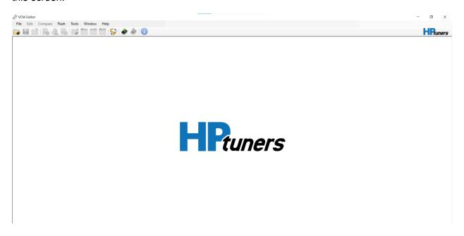
Using the "File" button at the top corner, open the tune file your tuner sent you (NOTE: If you are doing this for multiple revisions, ensure that you open the newest file and load to your vehicle)
