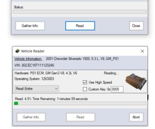
When the file is pulled, it will ask you to save a name to the file, be sure to use important characteristics like **Name**, **Vehicle**, and "**Base File**" so your tuner can designate.
